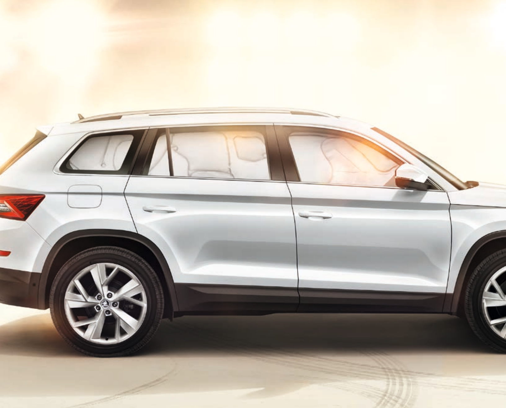
HEAD AIRBAGS Upon activation, head airbags create a wall protecting the front and rear occupants against head injury.
