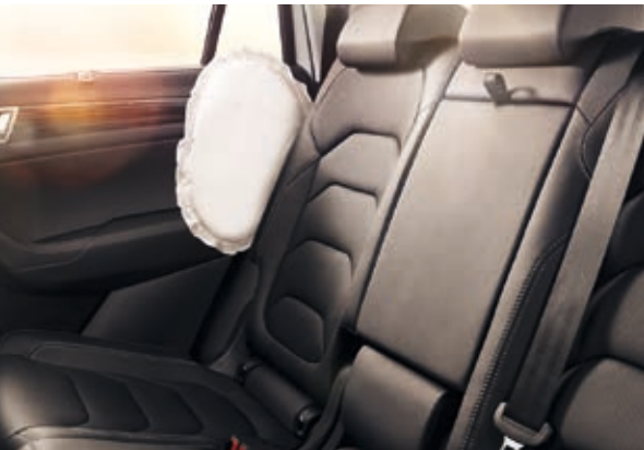
FRONT AND REAR SIDE AIRBAGS These four airbags protect the pelvis and chest of the driver and other passengers in the event of a side collision.
