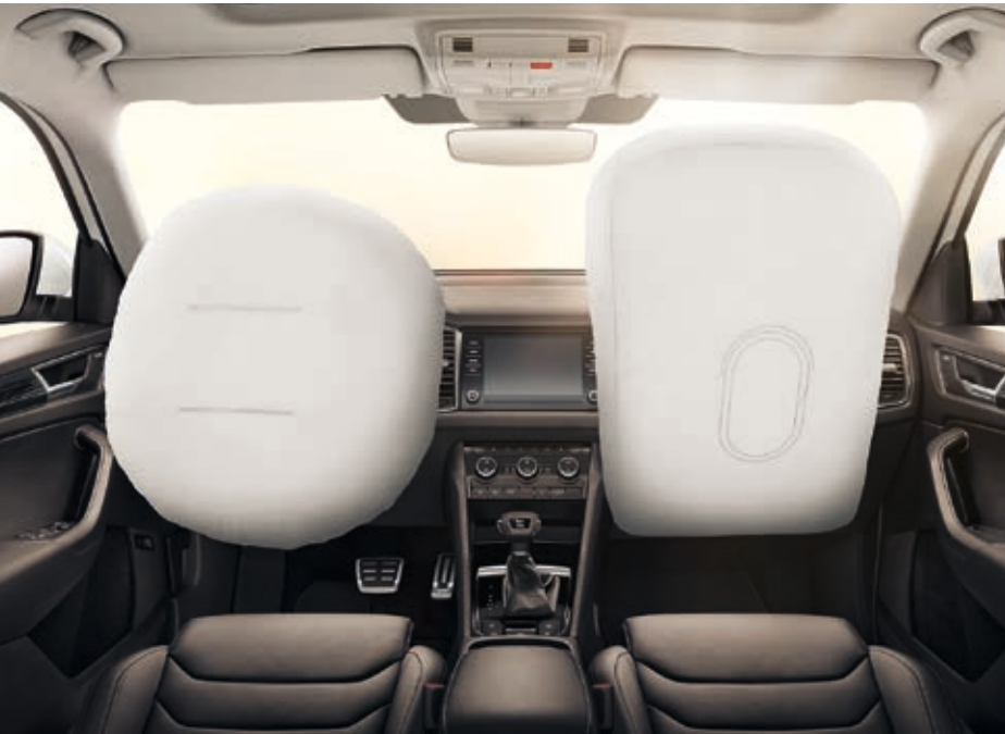
FRONT DRIVER AND PASSENGER AIRBAGS While the driver airbag is enclosed in the steering wheel, the passenger airbag is located in the dashboard. If needed, this can be deactivated when a child seat is installed on the front seat.
