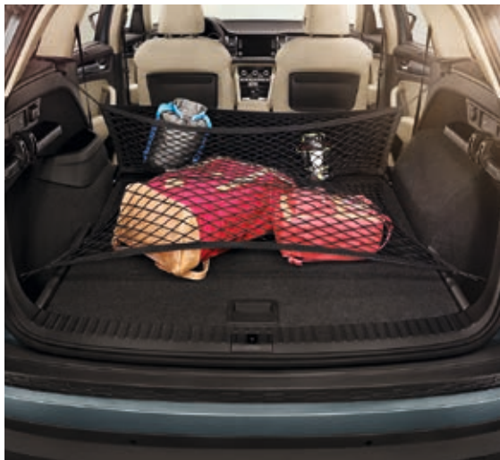
NET PROGRAMME One horizontal and two vertical nets increase the flexibility of the luggage space while firmly securing objects.
