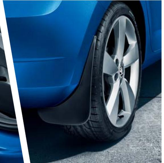
Rear mud flaps protect the chassis from mud and flying stones.
