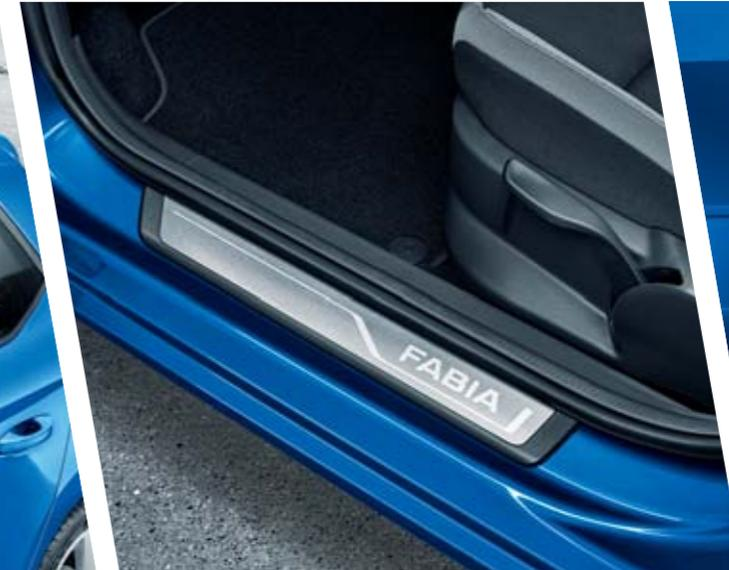
Decorative door sill covers with aluminium inserts underline the car's unique design, besides protecting the door sills against mechanical damage.
